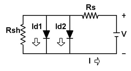
$$Y = K3* \left[ P1* \left\{ \begin{array}{c} \left[ \frac{K1*(Y/K3-X*P5/K4)}{(273.15+K2)} \right]_{-1} \\ + X*P5/K4 \\ -P3* \left\{ e^{\left[ \frac{K1*(Y/K3-X*P5/K4)}{(P4*(273.15+K2))} \right]_{-1} \right\}} \right] \\ \end{array} \right]$$
